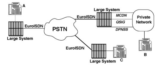
Figure 50: Remote user B or C is in the system private network
