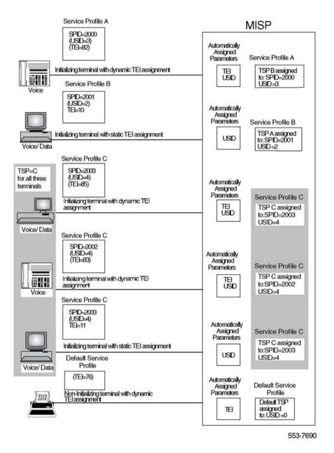
Figure 27: Terminal initialization and service profile assignment examples
