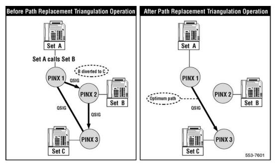
Figure 97: Triangulation Path Replacement
