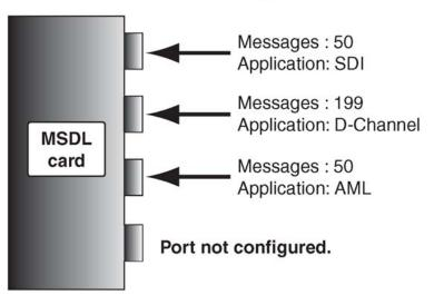
Total Messages per two seconds = 50 + 199 + 50 = 299 messages. 300th message arrives through port 1, it triggers a port overload check. On detection of a port overload, the port is locked; the incoming message count of the card is reduced by 200, bringing the card mesasge count to 100 (50 SDI + 50 AML).
