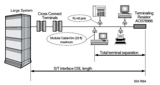
Figure 22: Extended passive SILC DSL
