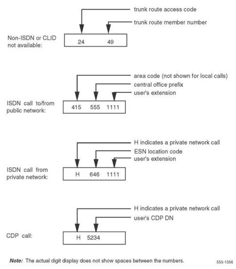
Figure 78: Digit display format for Calling Line Identification
