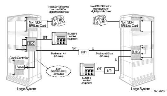
Figure 11: ISDN BRI TIE trunk connectivity - second configuration
