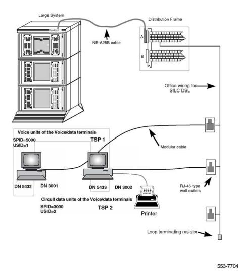
Figure 28: DSL terminal configuration
