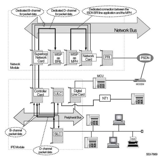
Figure 7: Packet data transmission using the MPH
