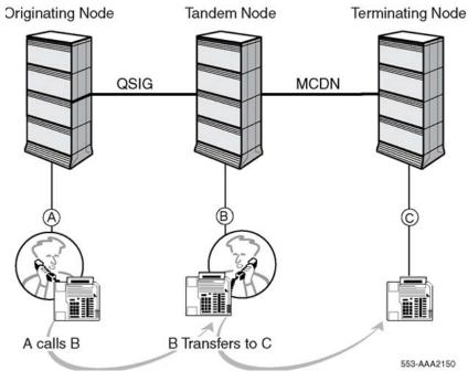
Figure 93: Call Transfer over a QSIG/MCDN link
