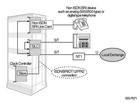
Figure 9: ISDN BRI trunk access for local exchange connectivity
