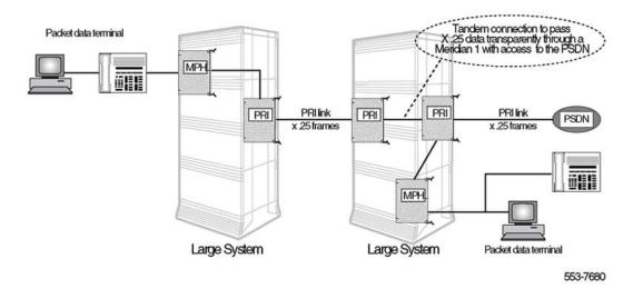
Figure 18: Tandem connections with the MPH
