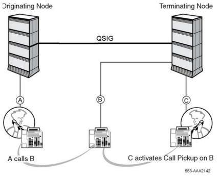
Figure 84: Call Pickup over a QSIG link
