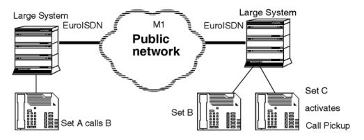
Figure 56: Call Pickup in a EuroISDN network
