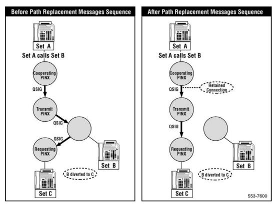
Figure 99: Path Replacement Retaining Part of Old Connection
