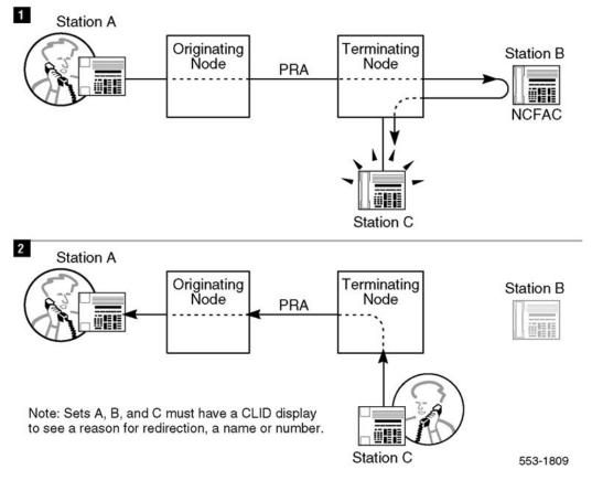
Figure 111: NCFAC intranode redirection
