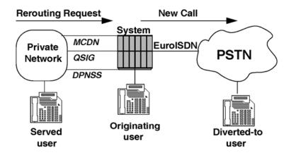
Figure 40: Rerouting request received at the originating node.
