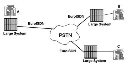
Figure 49: Remote user B or C is in a system private network
