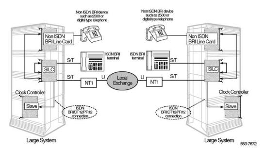
Figure 30: ISDN BRI TIE trunk configuration
