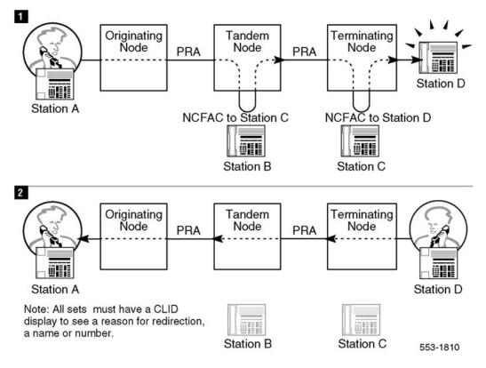
Figure 114: Tandem NCFAC intranode
