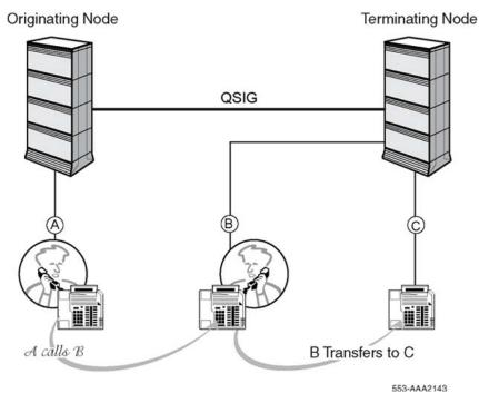
Figure 85: Call Transfer over a QSIG link
