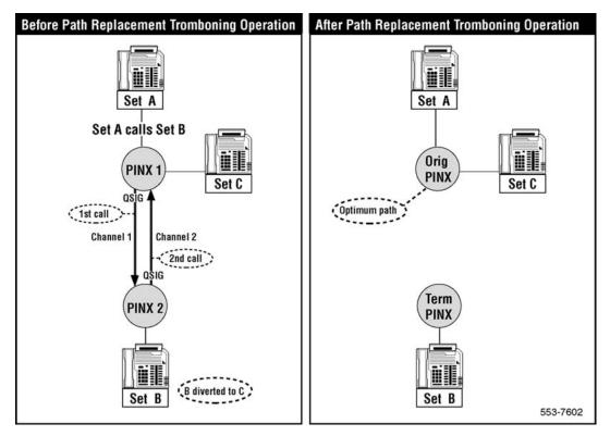
Figure 98: Tromboning Path Replacement
