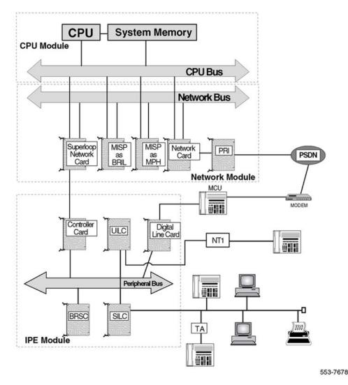
Figure 16: A basic ISDN BRI MPH packet data architecture, with a BRSC and an MCU
